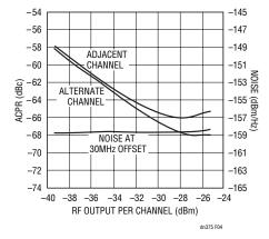
Figure 4. LT5528 4-Channel WCDMA Adjacent and Alternate CPR Measurement vs Channel Power
