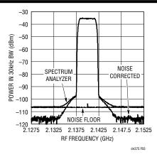
Figure 3. ACPR Spectrum for a Single Carrier WCDMA Signal
