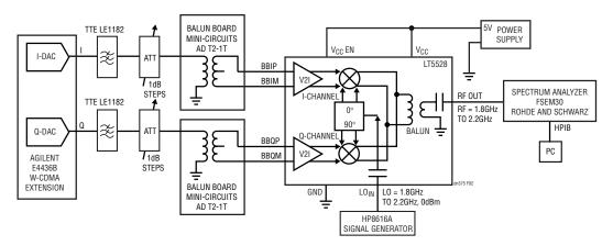
Figure 2. ACPR Measurement Setup
